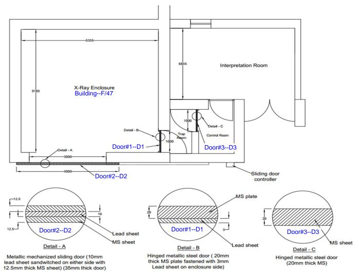
Figure 1 : Schematic diagram of 3 Doors (D1, D2 & D3)—Location & cross sectional detail
