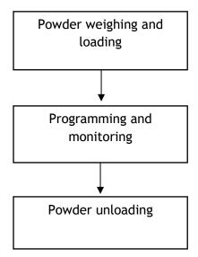
14. Process flow chart for sample preparation for hot pressing/diffusion bonding
