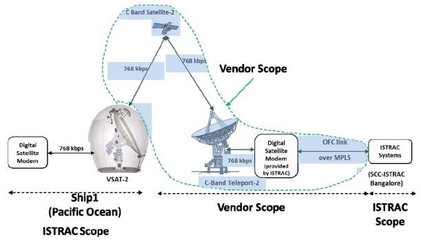
4.2.3 Circuit-3 (Hybrid Communication link from Ship-2 to MOX-ISTRAC)
