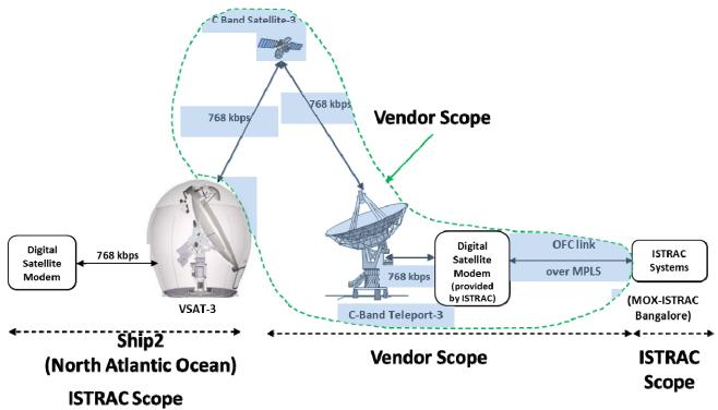
4.2.4 Circuit-4 (Hybrid Communication link from Ship-2 to SCC-ISTRAC)
