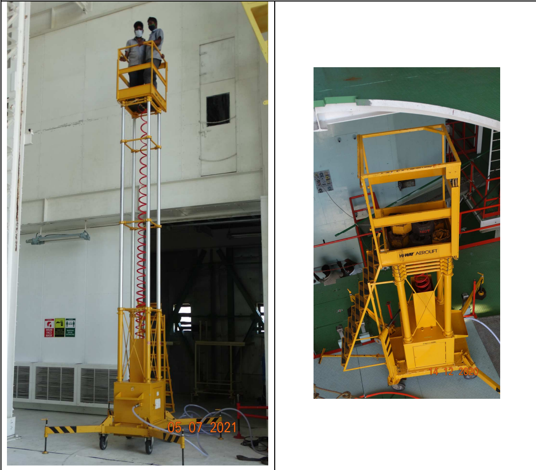
Four mast type Aero lift in raised and stowed condition (for reference purpose only)
