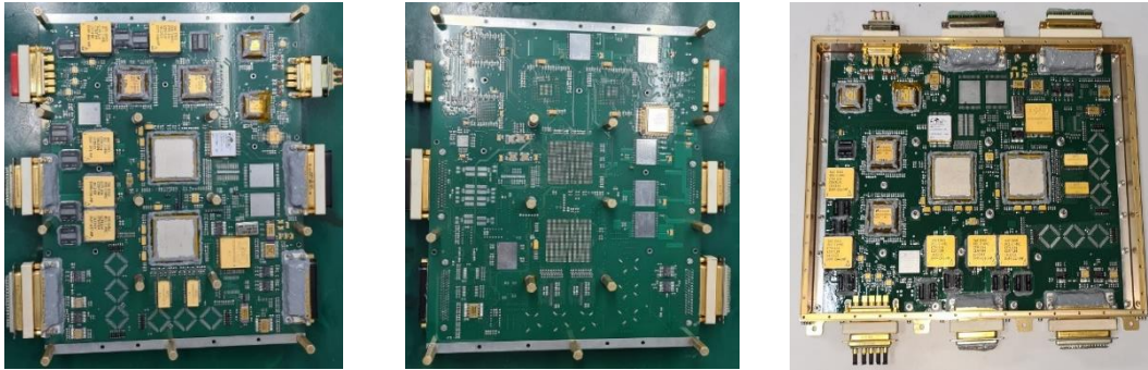
Figure 2. Top and Bottom views of the DPU PCB, PCB in Housing
